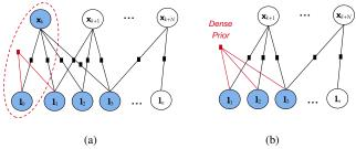
Fig. 3: (a) represents the full-size sliding window, the variables that need to be marginalized (dotted red) and the current prior (red). The states in the MB of this marginalization clique are represented in blue. (b) represents the effect of marginalization on the factor graph: the dense prior factor is updated.
