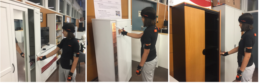
Fig. 5 Demonstrations were recorded using an Xsens MVN motion capture system. The teacher opens three doors with different radius.
