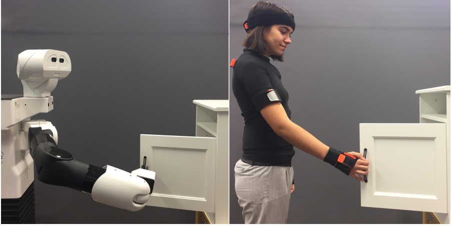
Fig. 1 The Gaussian-Process-based LfD approach allows to teach robot tasks such as opening doors.
